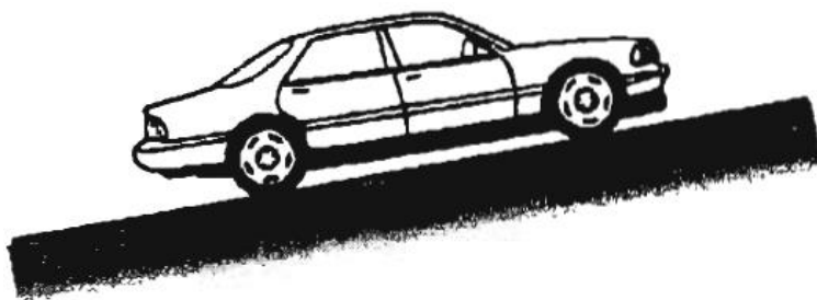
Figure 21.6 Gain of potential energy by an electric automobile going uphill.
